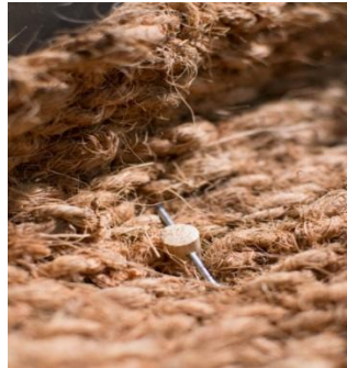
Coconut fiber geotextiles as beach revetment
